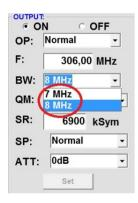
Choose bandwidth depending on output frequency between 7 MHz and 8 MHz
