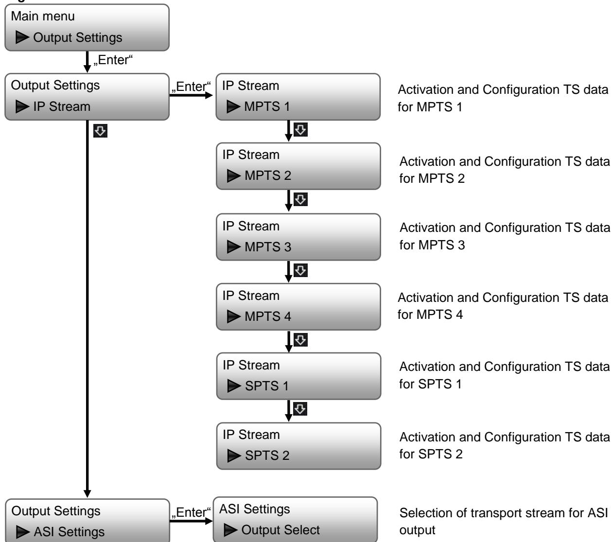
The signal of the ASI output ASI OUT 1 is also mirrored at the ASI output ASI OUT 2. The transport streams MPTS 1, MPTS 2, MPTS 3, MPTS 4, SPTS 1 or SPTS 2 can be selected as the ASI output signal.
