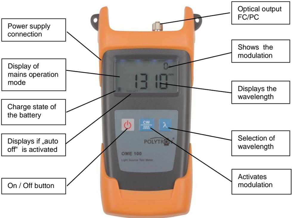
⏻ On / Off – Button: Switches the device on or off.
