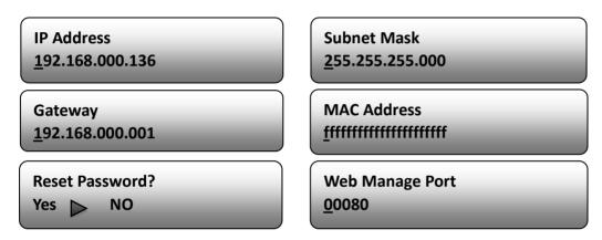
NOTE: The MAC address is according to the factory setting, and it is unique.
