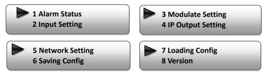
User can press UP/DOWN buttons to specify menu item, and then press ENTER to enter the submenus as below:
