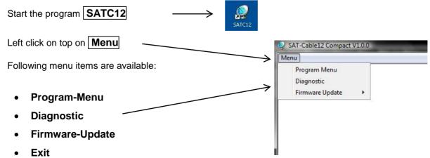
In "**Program-Menu**" all settings of input and output parameters are made. After calling the menu each of the 16 channels are retrieved and the *corresponding parameters settings* are displayed.
