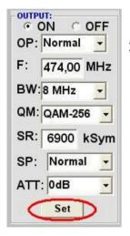
After setting all the parameters press the **Set** button. With this all the settings will be accepted. Repeat steps for other operating channels.
