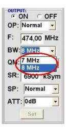
Select bandwidth according to output frequency between 7 MHz and 8 MHz
