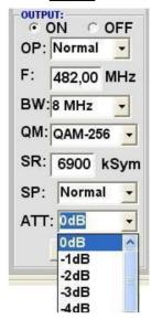
The output level at the output is 90dBµV and for each channel can be attenuated to 12 dB in 1dB steps.
