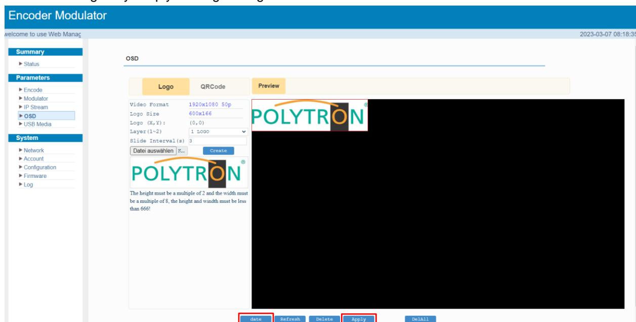
The time for displaying the logo must be precisely defined. To do this, press the "date" button and the following setting menu will be opened. In this menu the definition of different time intervals for displaying the logo can be set.
